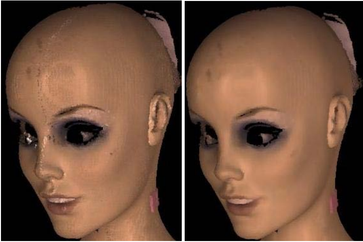
Fig. 4. Color cleansing of the Mannequin dataset - before (left) and after (right) modification of the lightness component in the HLS color space using a median filter
