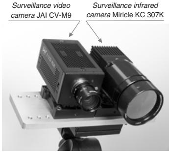
Fig. 4. A setup of a pair of video and infrared cameras for surveillance
