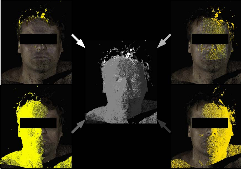
Fig. 7. Registration of partial scans: In this example, four partial scans of the frontal head are registered into a combined model. The different gray shades of the central image visualize the contributions of the different partial scans.
